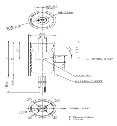
Note: Dimensions from an anode shank to a mounting hole.
