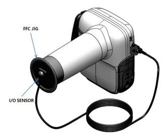
In order to obtain a low-noise image, execute the FFC (flat filed correction) function by using the FFC JIG provided for the first connection with the PORT-X IV and Intra Oral sensor
